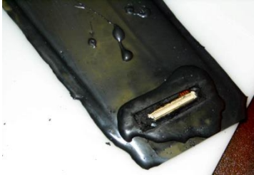
Sealant removal for data acquisition
