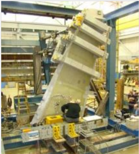
Northrop Grumman Full-Scale Testing of EA-6B Outer Wing Panels 2
